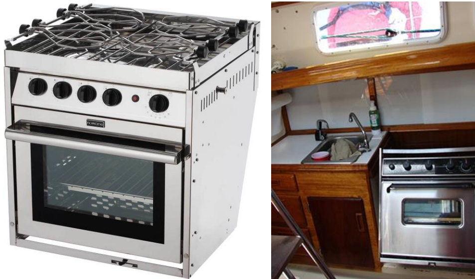
Figure 9. Gimbaled stove on sailboat remains vertical while boat heels. (Burden. 2019)
